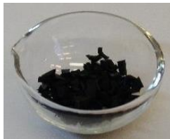
Conductive polymer composite by solvent process
